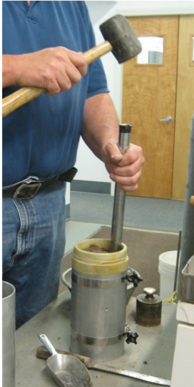
Figure 24. GeoTesting Express compaction process using a wooden dowel, rubber mallet, and split mold (photo courtesy of Nancy Hubbard)
