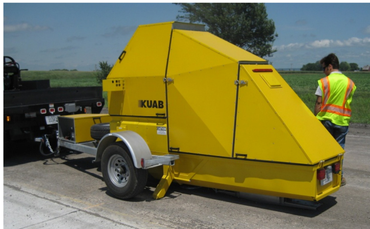
Figure 27. Falling weight deflectometer (FWD) in use on a concrete pavement surface
