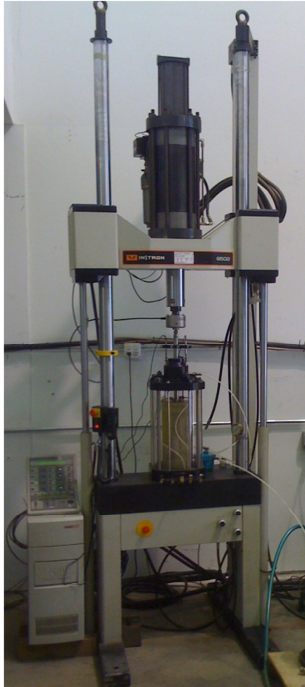
Figure 23. Boudreau Engineering, Inc. resilient modulus test equipment (photo courtesy of Rick Boudreau)
