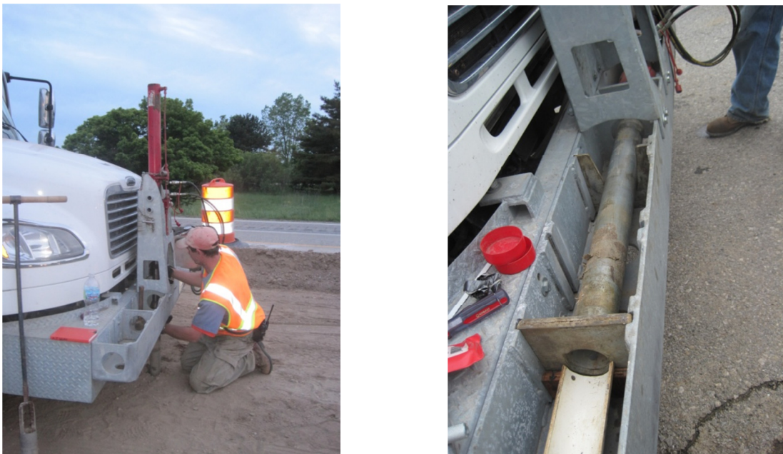
Figure 7. Shelby tube sampling; subgrade sample retrieval (left), sample extrusion (right)
