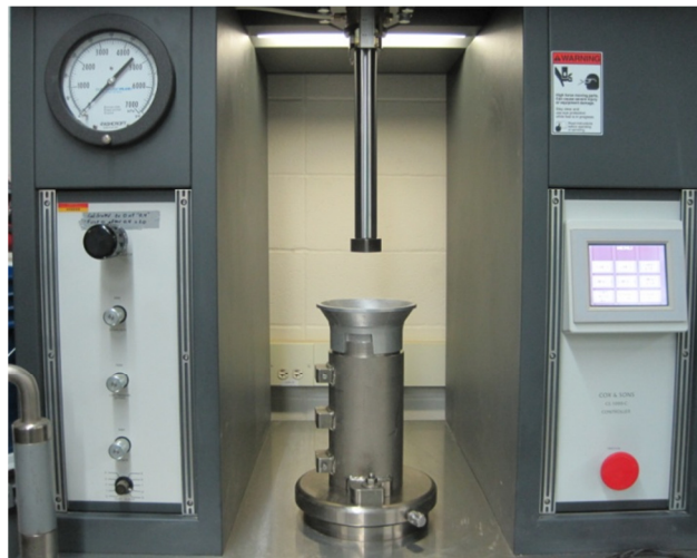
Figure 8. Cox and Sons kneading compactor used for cohesive soils
