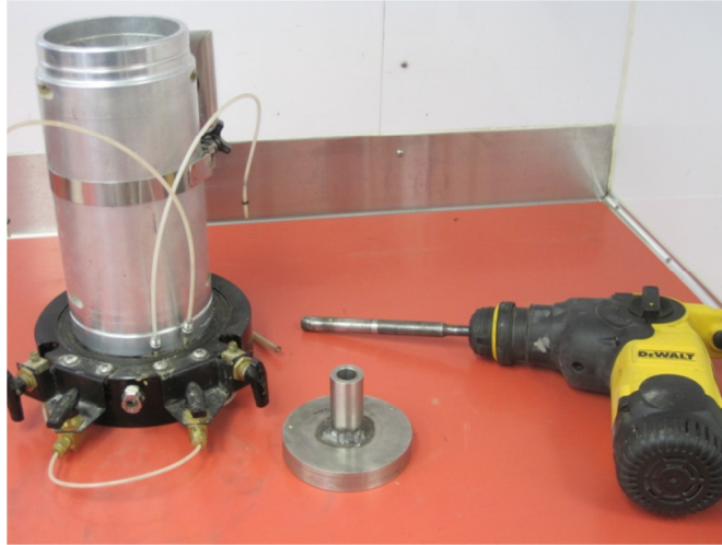
Figure 14. Split mold, steel platen (4 in. diameter), and vibratory hammer for compaction of granular materials
