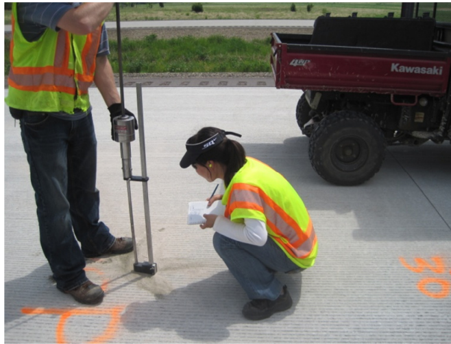
Figure 4. A dynamic cone penetrometer (DCP) in use
