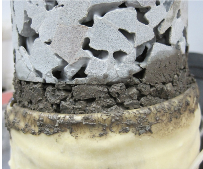
Figure 70. Pennsylvania US-22 composite material sample of CTB over class 2A subbase after M_r testing
