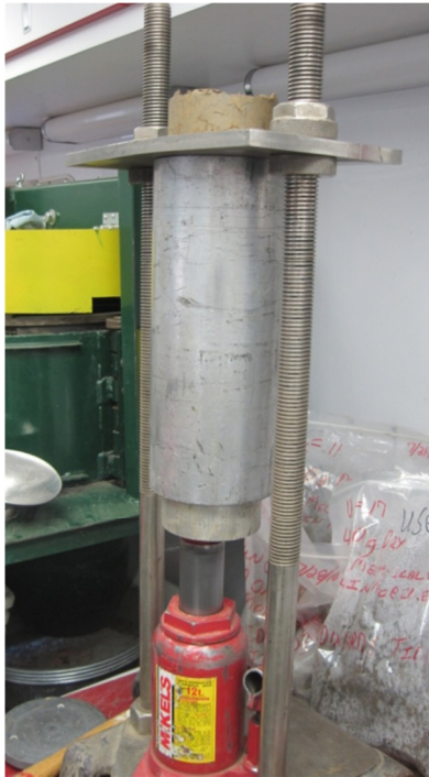
Figure 13. Extruding a statically compacted specimen
