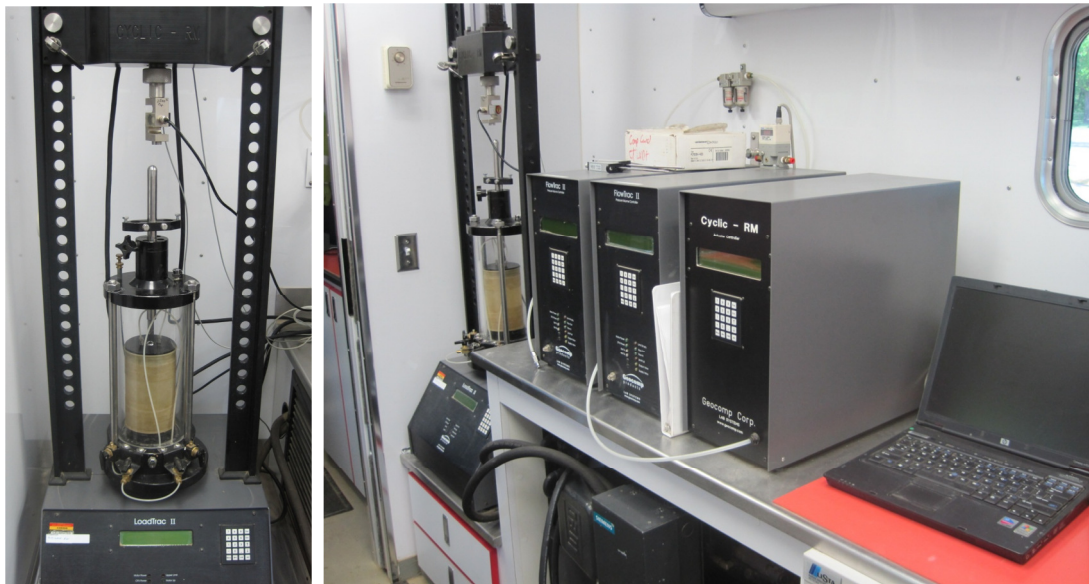
Figure 22. Triaxial chamber, load frame, and computer equipment for performing resilient modulus tests
