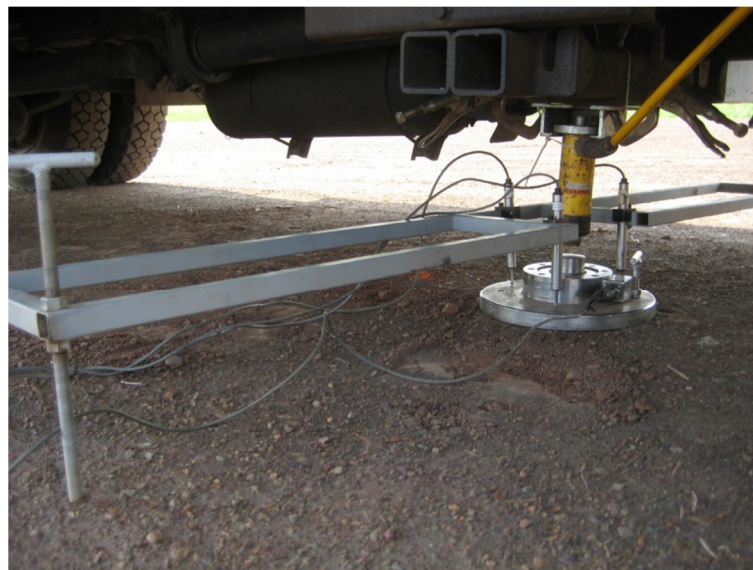
Figure 5. Plate load test (PLT) performed on subgrade
