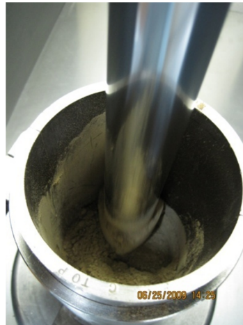
Figure 9. Soil compacted by kneading tamper foot
