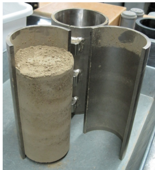
Figure 10. Compacted sample being removed from a 4 in. diameter split mold
