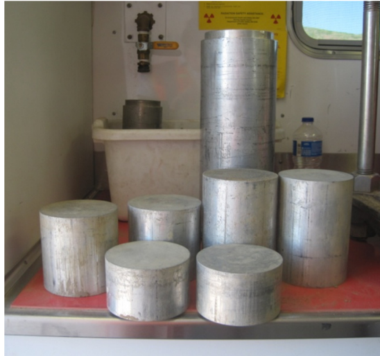
Figure 11. Aluminum spacers (4 in. diameter) used during static compaction
