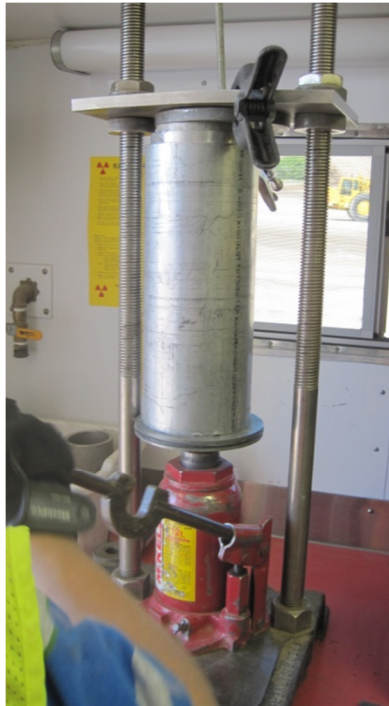
Figure 12. Static compaction of a cohesive specimen
