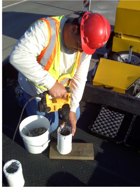
Figure 20. Compaction of OGS+HDP sample in the field
