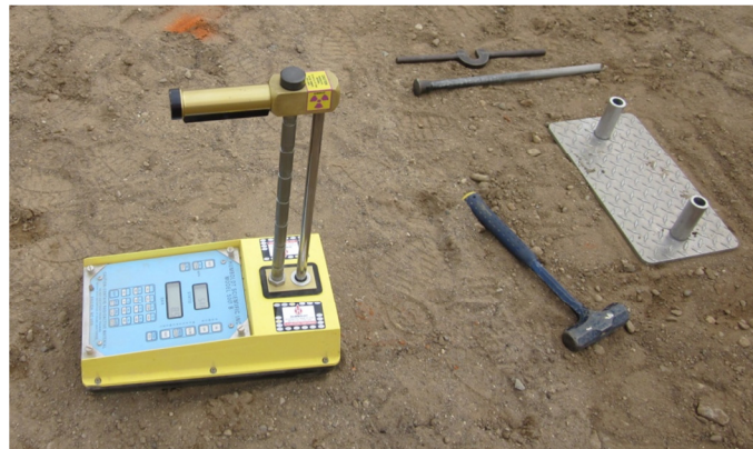
Figure 28. Nuclear moisture-density gauge with auxiliary equipment
