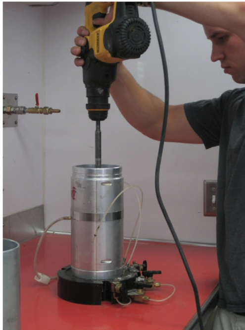
Figure 15. Compaction of granular materials in split mold
