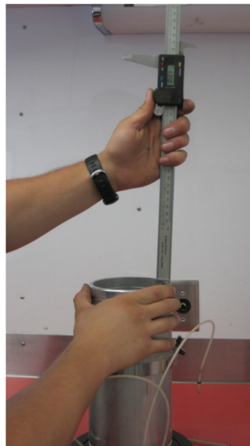
Figure 16. Verifying the thickness of each compacted layer with calipers
